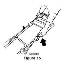
4. If the mower does not start in 1 or 2 pulls (or within 5 seconds using the electric starter), press the primer button 1 or 2 times and try starting it again.
